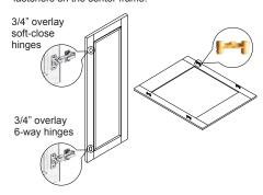
**Step 5:** Connect the doors to the box, hinges on the door panels snap into the hinges on the side panels. Insert the male fasteners into the female fasteners to attach the center frame.
