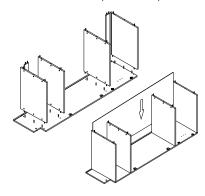
**Step 3:** Install the other side panel and toe kick using cam locks and wood dowels.
