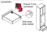
**Step 8:** After that, a small lever on the drawer front connector can be used to make small adjustment to correct clearance. Check the stability of the cabinet and make adjustment by tightening the cam locks.
